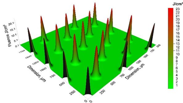
Fig. 1. Fluence distribution in the treatment plane on the skin surface. Treatment spot size 6 mm, peak fluences are 23 J/cm<sup>2</sup> and average fluence setting 0.71 J/cm<sup>2</sup>.
